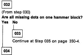
Exchange the hammer bank (MIM 300-1, "Hammer Bank") if the printer has a linac (early level) hammer unit or exchange the hammer block (MIM 300-1, "Hammer Block") for a printer with a clicking (late level) hammer unit.
