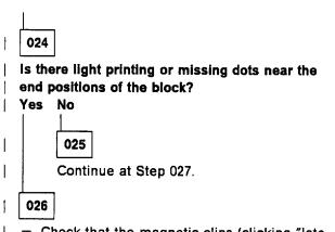
Check that the magnetic clips (clicking "late level" hammer unit only) are installed correctly.
