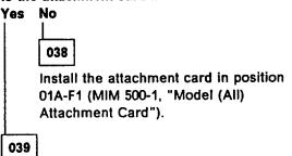
The printer logic is sensing that the attachment card is not installed. Reseat the attachment card and recheck the symptoms (MIM 500-1, "Model (All) Attachment Card"). If the same failure is still present, exchange the following, one at a time:
