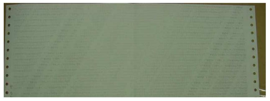
The above picture shows banding. Note that one line starts out dark on the left side and transitions to light towards the right. The next line starts out light on the left side and transitions to dark on the right. This repeats every other line. Do not be concerned about the lightness of the print in this picture. It is just to illustrate the "banding" effect.
