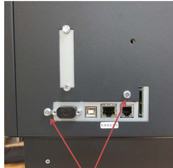
Two fasteners secure the I/O ports to the rear card cage wall.
